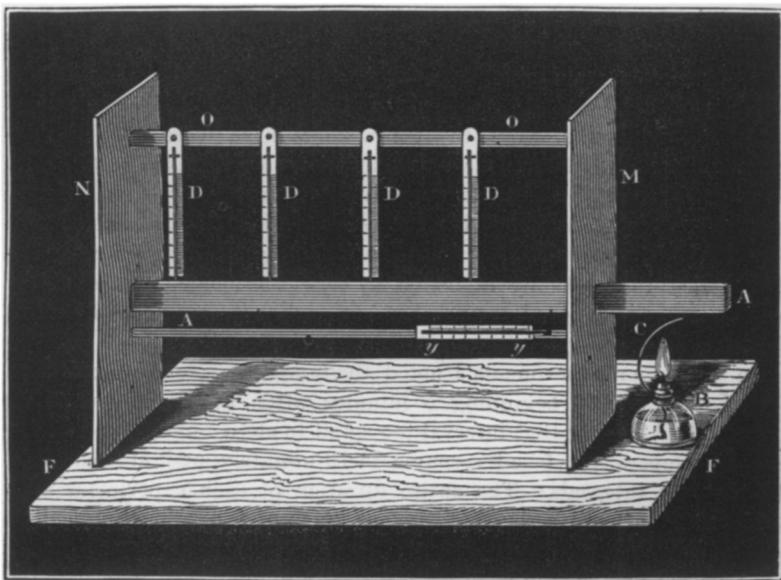
ratus shown in the diagram. It consists of a wooden baseboard (F F), 29 inches in length by 9 in breadth, on which are fixed two upright
